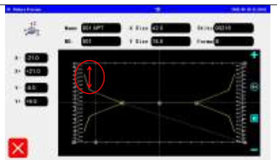
Cutting the middle point with a distance of 6 in the Y direction
