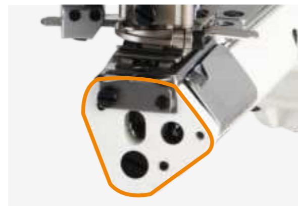
Small cylinder with 150mm circumference, which is smoother for sewing
