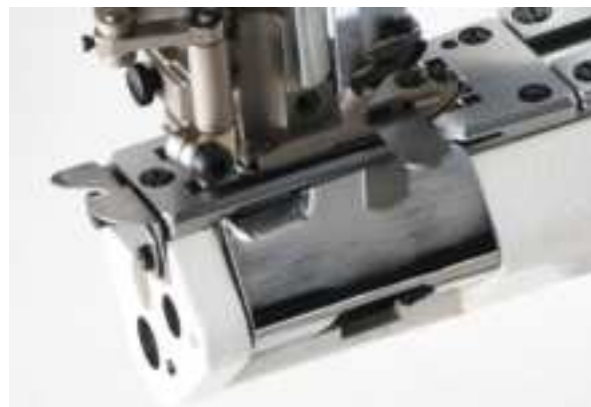
Spring-type presser foot structure, wide fabric adaptability
